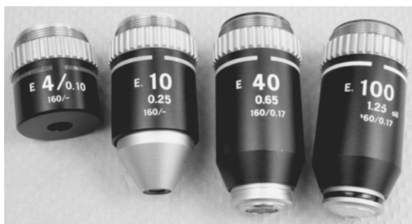
Figure 2. Objectives of the Nikon Alphaphot. The upper large numbers indicate the magnifying power of the objective; 4 - 100x. The number to the side or just below the mag. value indicates the numerical aperture of the objective; 0.1-1.25. The numbers at the bottom give some other information about the objective.
